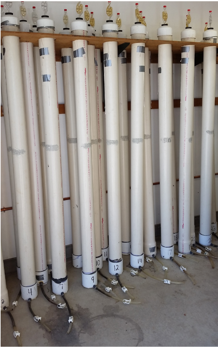
Figure 2. Effluent was drained and collected from the bottom of the ensiling tubes.
