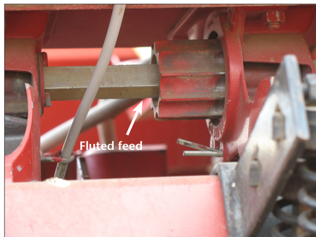
Figure 3. By modifying the fluted feed on his drill, Tom is able to achieve more accurate seed metering and placement.
