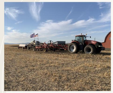
BOURGAULT 5710 3" BOOT, SINGLE ROW, ON 10" SPACING, SEMI-PNEUMATIC PACKERS
