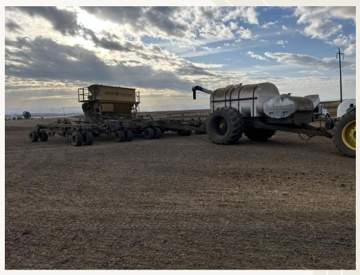
SEED MASTER 5010 PRECISION HOE ON 10" SPACING, INDIVIDUAL ROW PACKERS ON ISO HYDRAULIC CONTROL
